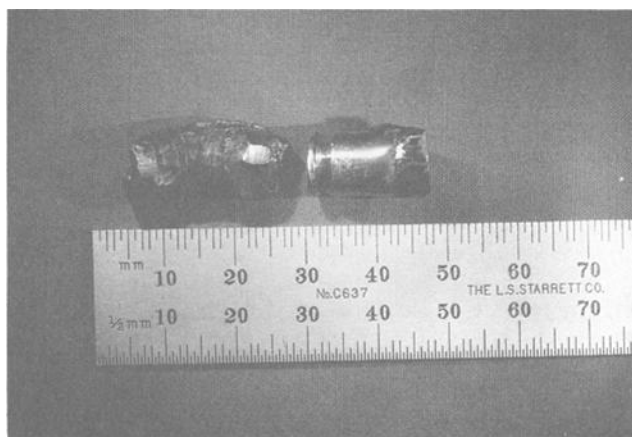
FIG. 3—Photograph of both projectiles showing the .44 caliber bullet that accelerated the cartridge case down the bore, coating its base with lead.
