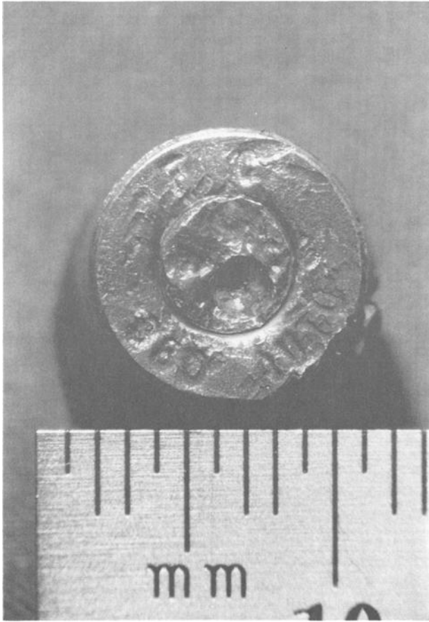
FIG. 4—Photograph of the base of the cartridge as an accessory projectile. The primer contains a firing pin impression, indicating its previous expenditure, while the base is partially obscured by the heavy deposits of lead from the bullet, indicating it was pushed down the bore. It does not show the marked deformation a bullet would make had the casing been an intermediate target.
